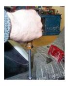
Remove the 2 lower screws located under the saddle with a screwdriver.
