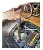
Remove the superiors screws from the cover located under the saddle with a cross-shaped screwdriver.
